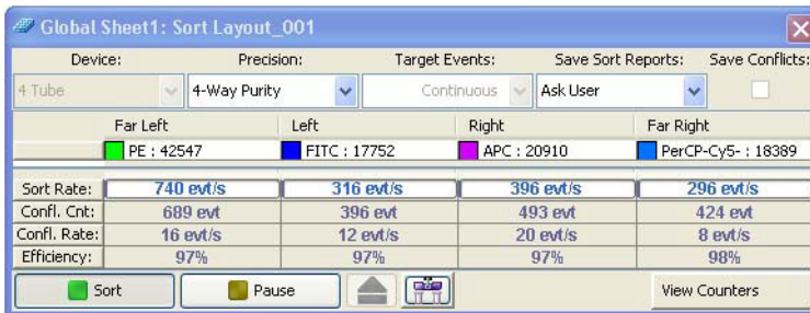
Figure 2-16 Sort layout for a four-way sort
