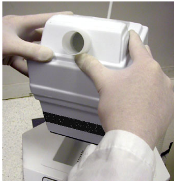
Figure C-8 Inserting the new filter
