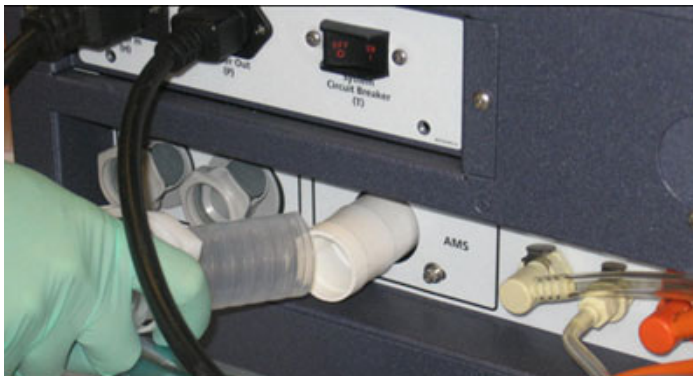
Figure C-6 Disconnecting tubing (side of instrument)
