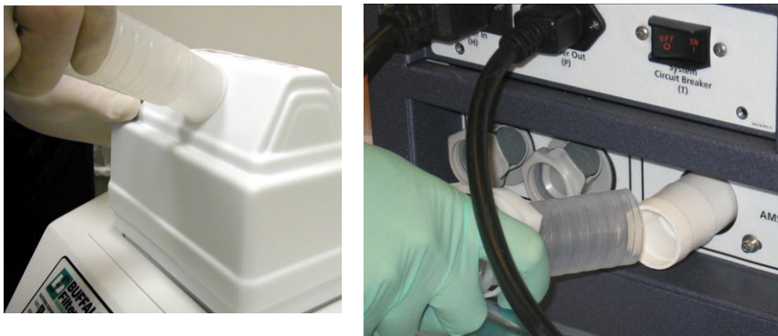
Figure C-10 Connecting new tubing
