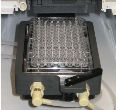
Figure 1-15 Plate Loader on ACDU
