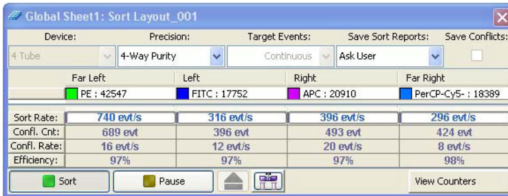
Figure 3-12 Sort layout during sorting
