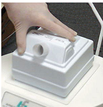
Figure C-9 Seating the new filter
