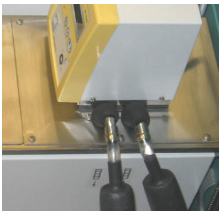
Figure D-2 Input and output ports on water bath
