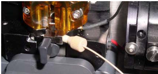
Figure 6-1 Closed-loop nozzle installed in flow cell
