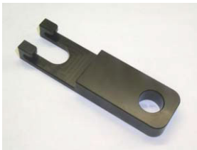
Figure 6-30 Deflection plate removal tool
