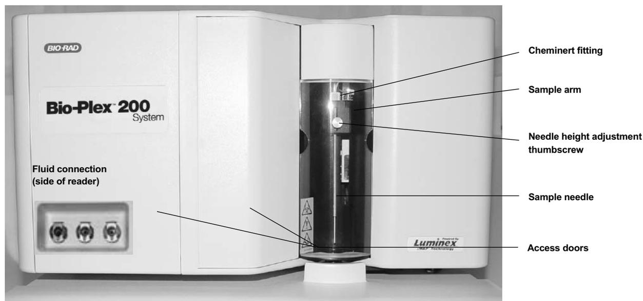
Fig. 1. Array reader – front and side panel features.
