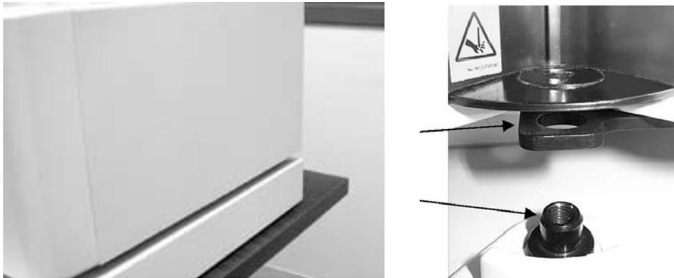
Fig. 10. Reader aligned on top of microplate platform.
